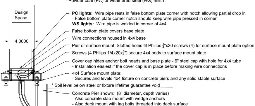
Conduit L  $(\frac{3}{4})$  routes wires to bollard base for pier mount
