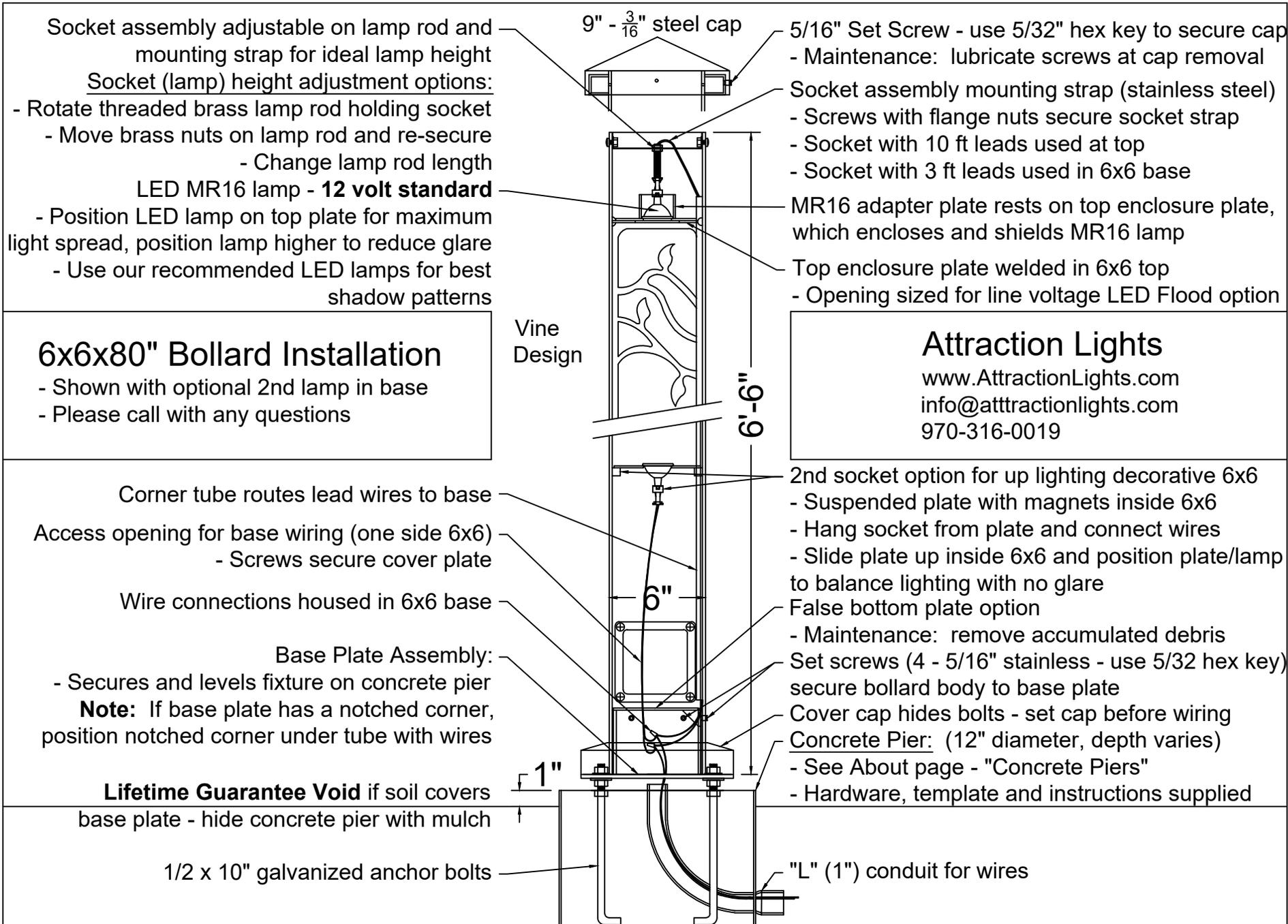
Socket assembly adjustable on lamp rod and mounting strap for ideal lamp height
