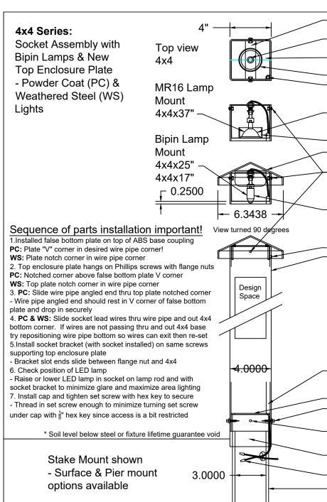
Stainless steel socket bracket supports socket for LED lamp
